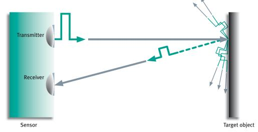
The times when the pulse was sent and received are measured extremely accurately.
